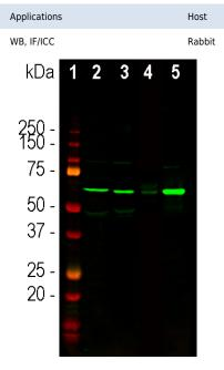
Western blot analysis of different tissue and cell lysates using rabbit pAb to TH, RPCA-TH, dilution 1:5,000 in green: [1] protein standard (red), [2] rat brain, [3] mouse brain, [4] SH-SY5Y cells, and [5] PC12 cells. The strong band at about 60kDa corresponds to TH protein expected in brain and PC12 extracts but not in SH-SY5Y cells.
